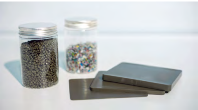
Pellets recycled from plastic bags (granules in the bottle on the left)
