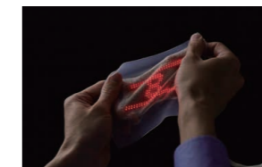
2018 Developed a stretchable thin display in collaboration with the University of Tokyo: Skin electronics device that attaches to skin
