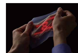
2018 Developed a stretchable thin display in collaboration with the University of Tokyo: Skin electronics device that attaches to skin
