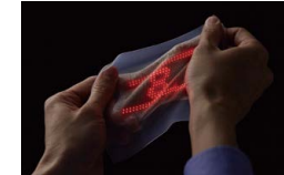
2018 Developed a stretchable thin display in collaboration with the University of Tokyo: Skin electronics device that attaches to skin
