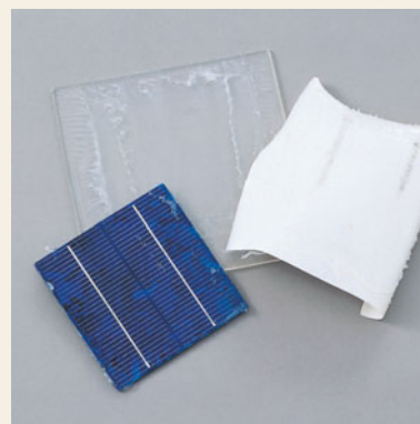
Detached solar battery (from left) cell, glass, filling sheet
