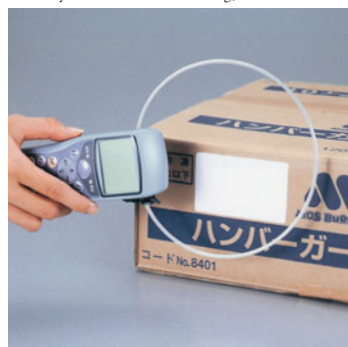
Delivery case labeled with IC tag, and reader
