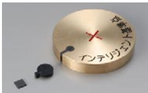
Intelligent control point containing IC tag
