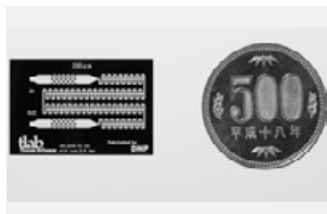
A micro flow channel chip compared to a 500-yen coin
