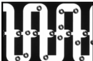
Glass pieces 100 \mu m in diameter trapped in flow channels
