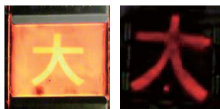
Various materials shine after light-emitting material is printed onto them Left: printed glass sheet Right: printed cloth
