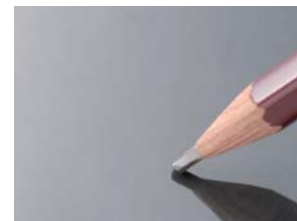
DNP's new hard-coat surface film resists pencil scratching
