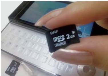
MicroSD card with MULTOS operating system
