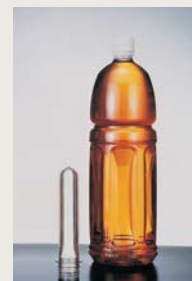
Left: preform, before being formed into bottle Right: PET plastic bottle after forming
