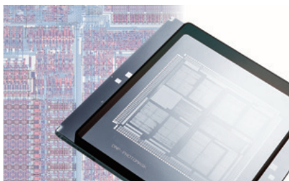
A photomask used for manufacturing semiconductors
