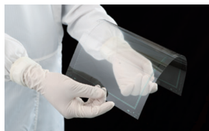
Electrode film for capacitive touch panels
