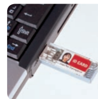
Yubi-net Pass Micro reader-writer for IC cards
