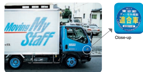
Regulation-compliant vehicle with particulate filter installed
