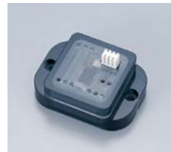
RFIDs containing heat, moisture, and light sensors
