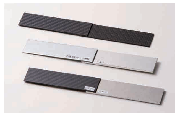
Bonding dissimilar materials such as aluminum and CFRP
