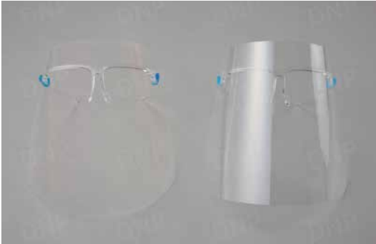
DNP ultra-low reflection face shield (left), for which we assessed durability against alcohol disinfectants, ultraviolet rays blocking rate and degree of damage when dropped
